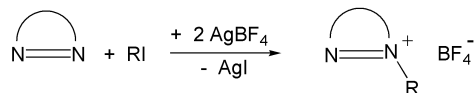
Scheme 2. Preparation of bicyclic examples of six-, five-, and four-membered ring diazenium tetrafluoroborate salts (R = alkyl).
