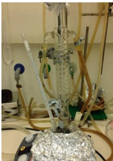
Figure 9. Etherification of glycerol in a reflux system.
