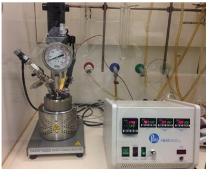
Figure 10. High-pressure autoclave reactor.
