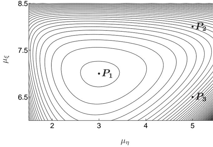
FIG. 3.3. Level sets of  $f(\mu_\xi, \mu_\eta)$  associated with the interior supporting eigenvalues for the sharp estimate in four-dimensional Krylov subspaces. The continuous minimum is attained in  $P_1 = (7, 3)^T$ . Although  $P_3$  is close to  $P_1$  compared to  $P_2$ , the function takes the larger function value in  $P_3$ .
