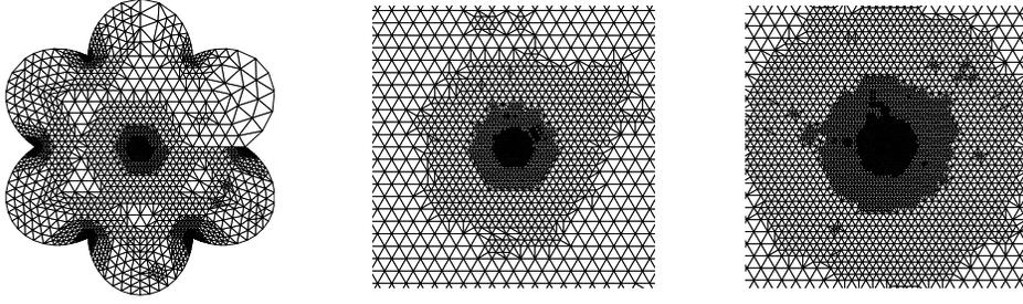
FIG. 4.2. Triangle meshes with 2,768, 69,118 and 676,518 nodes and associated numbers of 2,582, 67,870 and 672,500 inner nodes. The associated depths of the triangulations are 17, 38 and 51. Square-shaped sectional enlargements around the critical point  $(0, 0)^T$  are drawn for the two finer meshes. The side lengths of these enlargements are  $3 \cdot 10^{-4}$  and  $6 \cdot 10^{-7}$  respectively.
