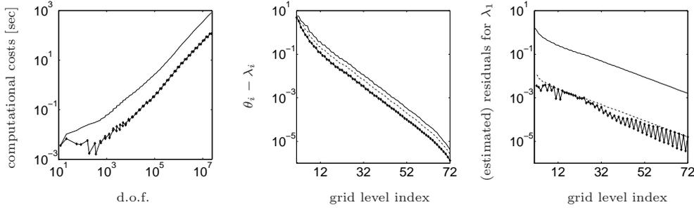
FIG. 4.3. Computational information on the AMP eigensolver for the approximation of the smallest eigenvalues by a block version of the restarted Krylov subspace iteration (1.3). Left: Cumulative computation times and computation times on the current level. Center: Convergence history of the eigenvalue approximations for the three smallest eigenvalues. Right: Error indicators of the residual-based error estimator associated with the smallest eigenvalue  $\lambda_1$ .
