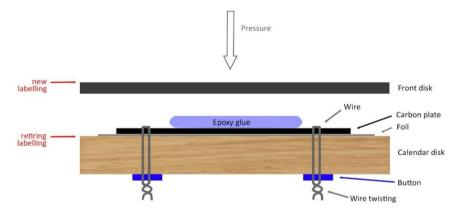
**Sketch:** The carbon plate (black) is tied to the inscribed side of the calendar disk with wires which are stuck through cracks in the disk and are twisted on the reverse side. Then, adhesive is applied to the carbon plate; a foil protects the historical inscription from excessive glue spilling sideways when the front disk is finally pressed down.
