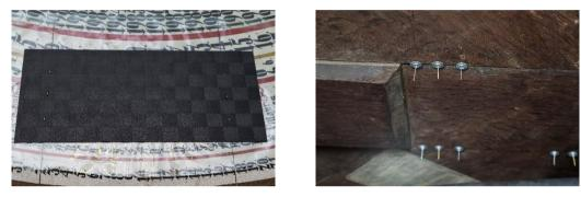
**Left:** One of the eight carbon plates on the calendar disk. Two groups of three wires each are visible. Each wire is passed through two drill holes and through gaps in the calendar disk. **Right:** On the rear side of the calendar disk, the wires go through buttons and are twisted to secure them in pace. Both pictures by Edeltraut Altrichter / ITMZ.
